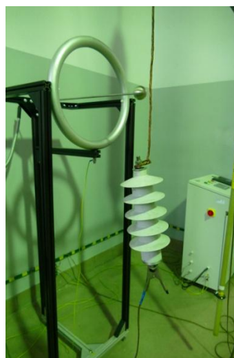
Fig. 4. Surge arresters during high voltage laboratory test
