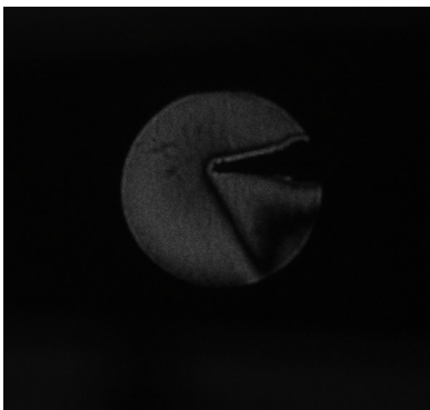
Fig. 7. Photograph of verification fringes due to concealed phase object is retrieved only when SH is perfectly repositioned.
