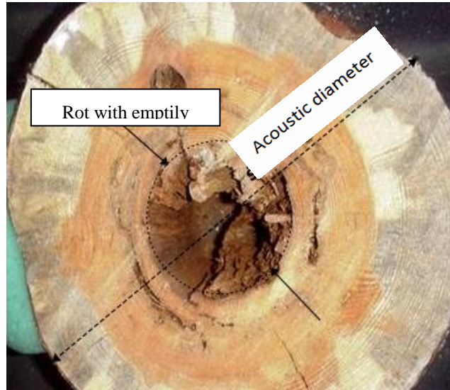
Fig. 7. Cross-sectional of wood with internal rot (sample with empty)
