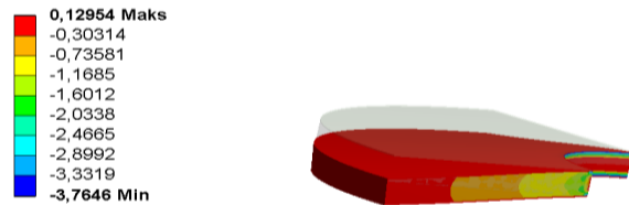
Fig. 3. Shear stress, linear core material – inner edge simply supported
