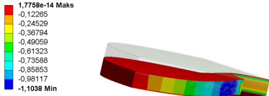
Fig. 5. Shear stress, nonlinear core material – inner edge simply supported
