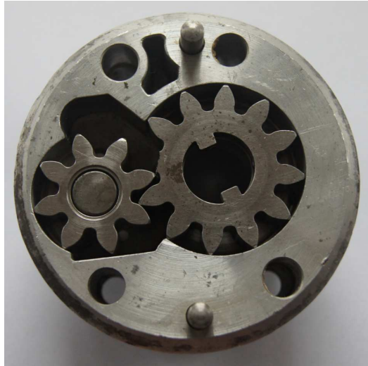
Fig. 1. Positive - displacement gear pump
