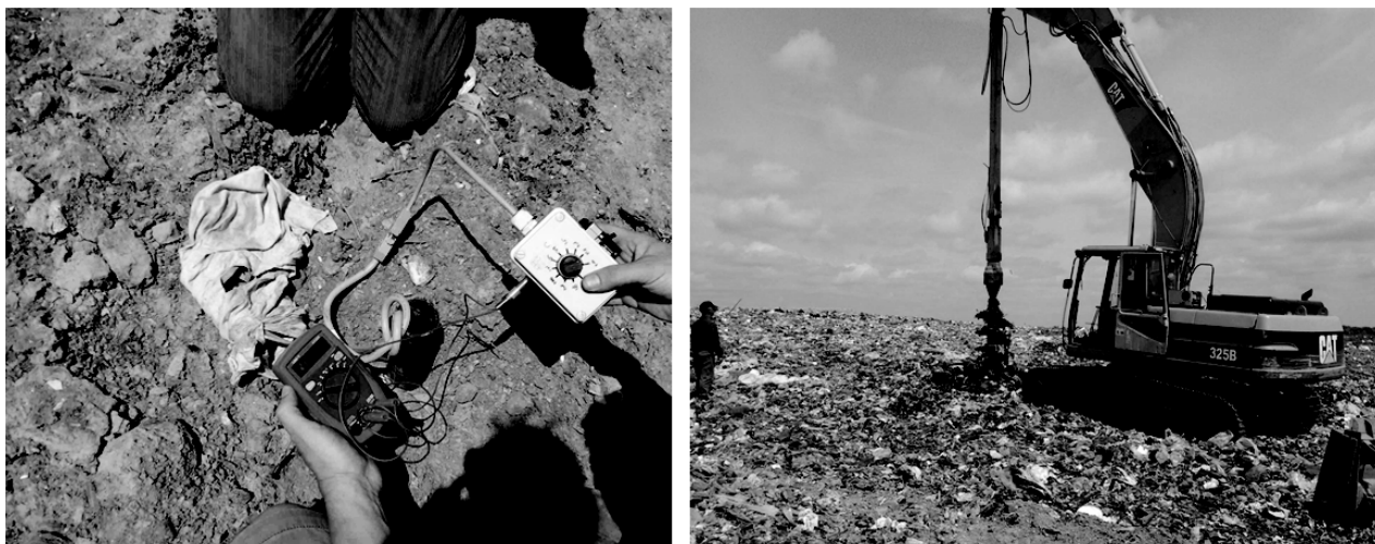
Fig. 4. Temperature reading at a monitoring well (left) and evolving of a borehole for installation of a temperature monitoring well (right)
