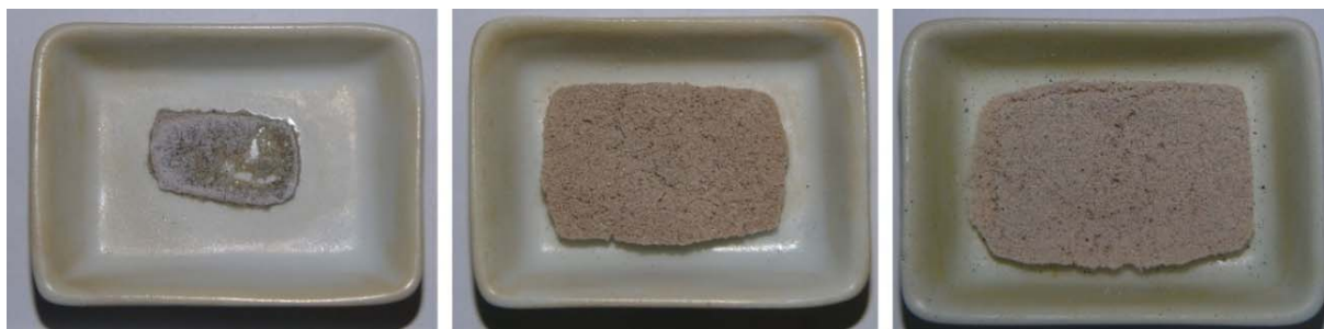
Fig. 7. Slag samples from cereal straw heated in the muffle furnace at the temperature of 1000°C, from the left: without additive, with Bolesław Śmiały coal ash and Turów lignite I ash
