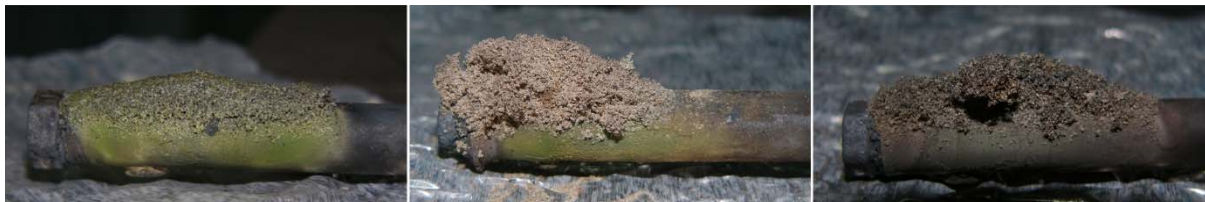
Fig. 10. Slag samples collected on the probe during biomass-firing, from the left: cereal straw, cereal straw with Turów lignite I ash and Bolesław Śmiały coal
