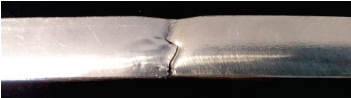
Fig. 7. A crack of specimen after static tensile test
