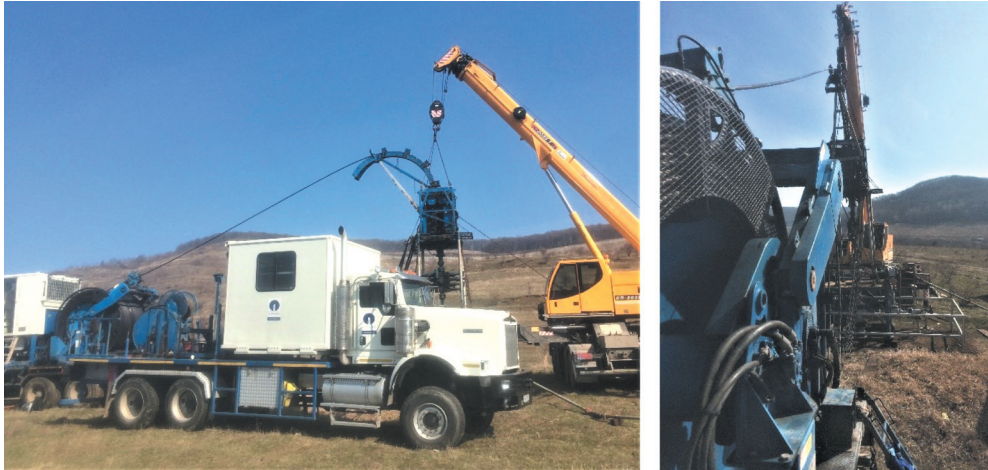
Fig. 5. Coiled tubing unit working on the field
