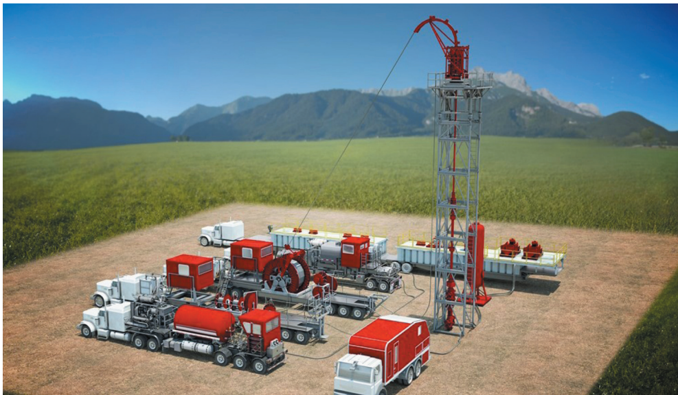
Fig. 2. Coiled tubing working scheme
