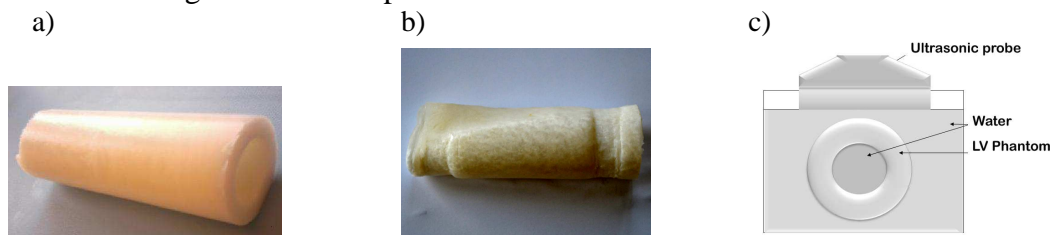
Fig.1. The LV models: a) – normal, b) with pathological change inside the wall, c) view of the cross-section of the LV model during examination.
