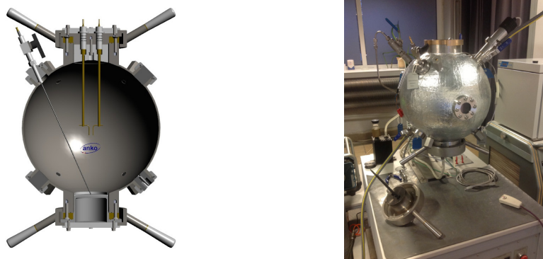
Figure 1. Experimental stand for testing flammability limits of fuel vapors
