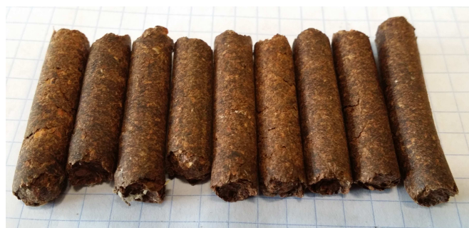
Fig. 6. View of pellets from onion skins obtained at a moisture content of 19.1%
