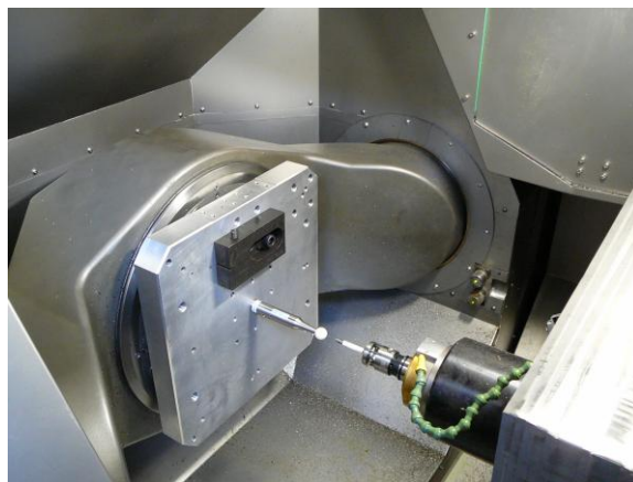
Fig. 4. Measurement of multi-directional errors of probes on the Nano-Focus machine. In the IPTAachen laboratory
