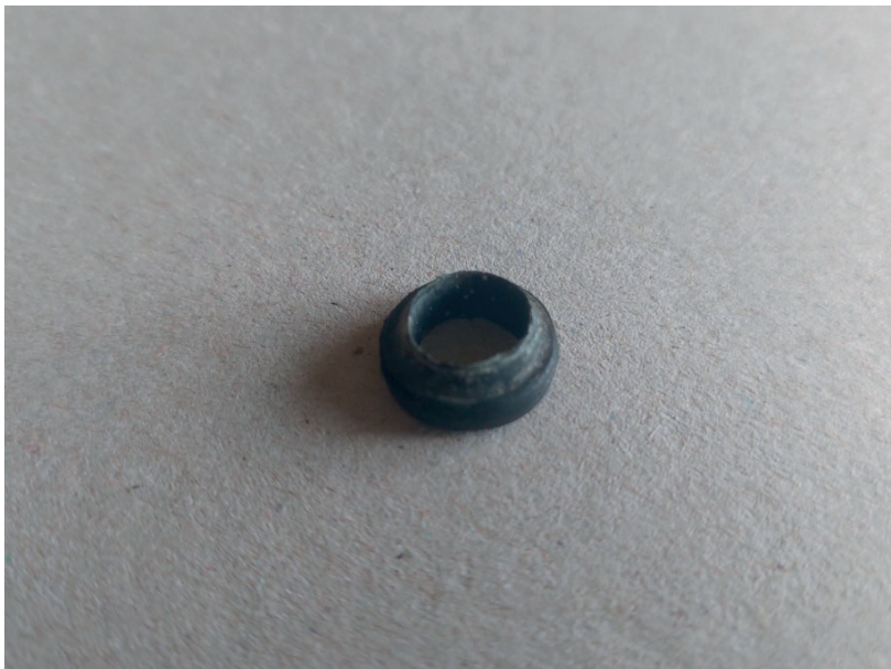
Fig. 6. Damaged rubber seal on a wash basin faucet, causing water leaks
