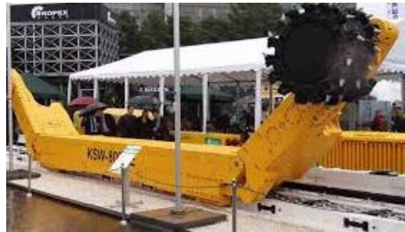
Fig. 7. KSW-800 NE longwall shearer [10]
