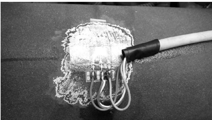
Fig. 7. Strain gauge in measure point T7
