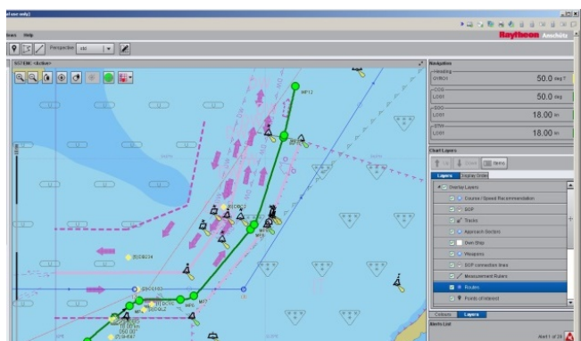
Figure 8. Project COSINUS results: Display of manoeuvring plan (green) of own ship together with route plan of another vessel (blue) presented in Integrated Navigation System of project partner Raytheon-Anschütz transmitted from VTS station of partner SIGNALIS
