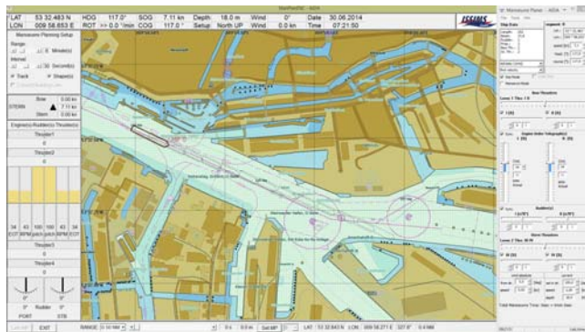
Figure 3. MP0 - Initial position: The prediction already shows that the ship would drift slightly to portside due to the set handle positions
