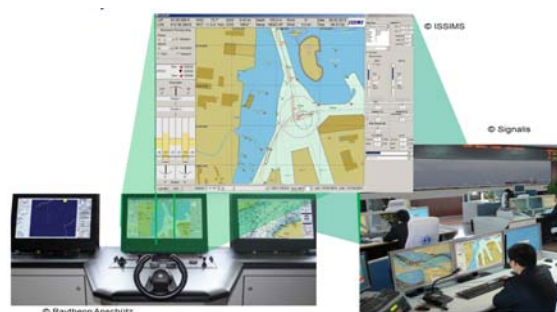
Figure 7. Project COSINUS – shared information on manoeuvring plans and multiple prediction in ECDIS between bridge and VTS
