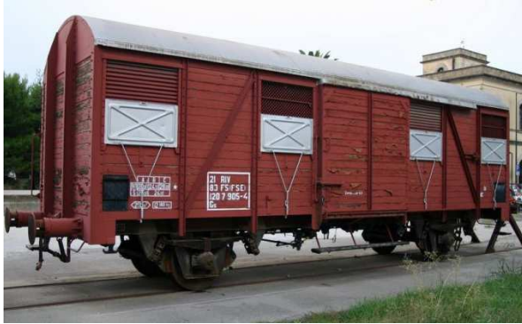
Fig. 3. Wagon type “GS” 12 Tons; in this and other similar wagons, after the '50s, beech plywood replaced the conventional painted European larch planking for the walls (Photo by Corrado Cremonini)
