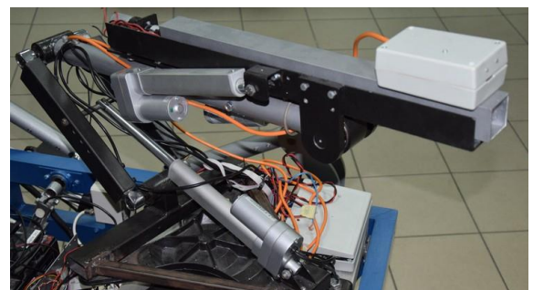
Fig. 8. Prototype of the manipulator on mobile wheel-legged platform
