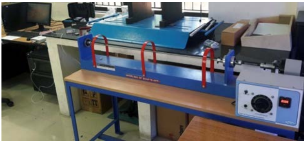
Fig. 1. Apparatus for measuring the bearing vibration data.
