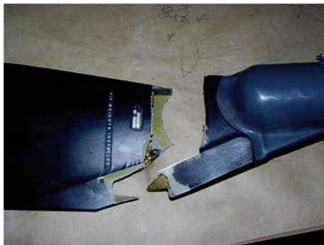
Figure 8. Robinson helicopter series main rotor blade crack caused by a fatigue process.
