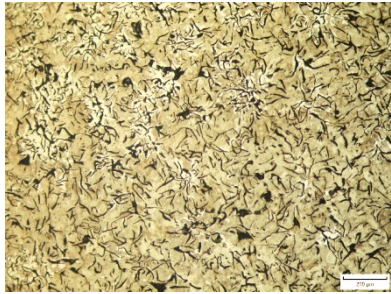
Fig. 7a: GJL 200 - cast state
