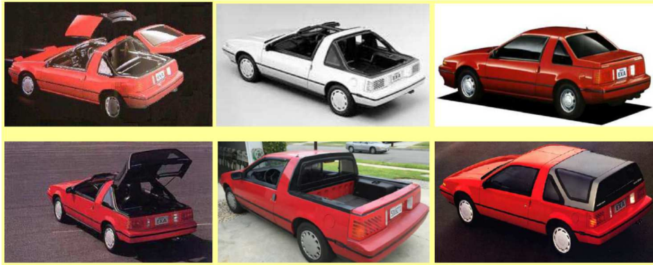
Fig. 4. Flexible control of spatial body architecture and functionality through modular styling approach: Nissan EXA 1990 vehicles range
