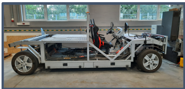
Figure 6a. A man-driven prototype platform equipped with the in-wheel DWH-200 motor. Source: Arex
