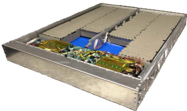
Figure 7. The interior of the BMU-200 battery module with a maximum capacity of 15 kWh, operating voltage of 600 V controlled by a bi-directional DC/DC converter with a load capacity of up to 30 kW. Source: Arex
