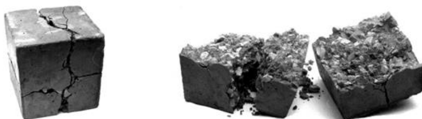
Figure 4. Example of a concrete specimen damaged by impact.
