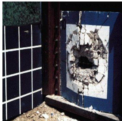
Figure 1. Investigation of concrete slab under the influence of explosion: a – view of a destruction plane of a plate in a special room, b – fragment of destruction.
