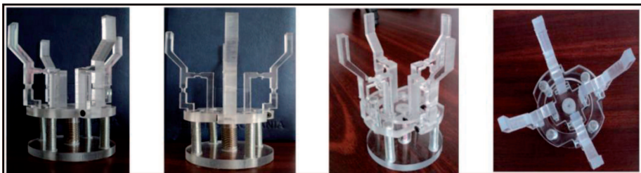
Fig. 5. The obtained compliant mini-gripper
