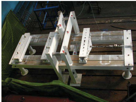
Fig. 3. Test stand lining mesh [2011]
