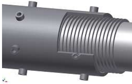
Figure 2: Geometry of the seal.
