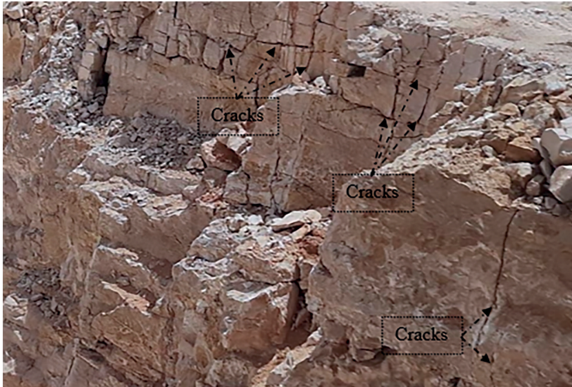
Fig. 4. State of the rock mass of the quarry
