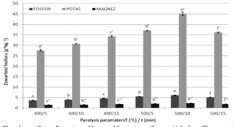
Legend: Fosfor: Phosphorus, Potas: Potassium, Magnez: Magnesium, Zawartość fosforu: The content of phosphorus **Fig. 2**. The content of phosphorus, potassium and magnesium in biocarbon obtained from rye straw depending on the pyrolysis parameters (temperature, time). Various letters indicate statistically significant differences between average values within group x, x', x'' (for  $p \le 0.05$ )
