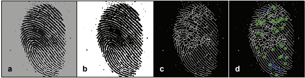
Fig. 9. Results of algorithm based on histogram alignment [12]. Filtered image (a), binarized form (b) and thinned form (c) with marked minutiae inside ROI (d).
