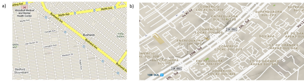
Figure 1: TN structures with a mesh topology (a), and routes with a tree-like structure in the city of Brasilia (b)
