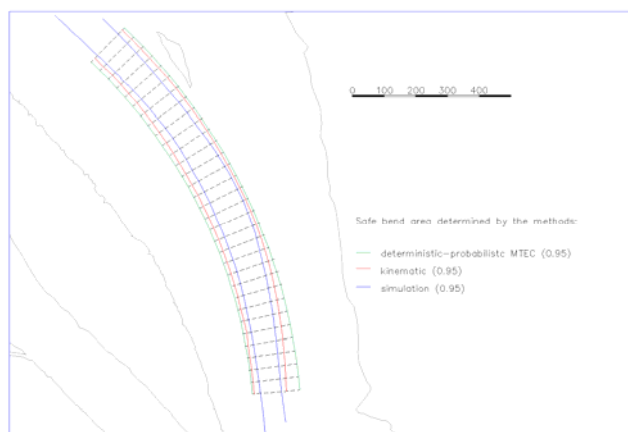
Figure 7. Safe width of the Ińskie bend, Świnoujście-Szczecin fairway, determined by the kinematic, simulation and deterministic-probabilistic MTEC methods.
