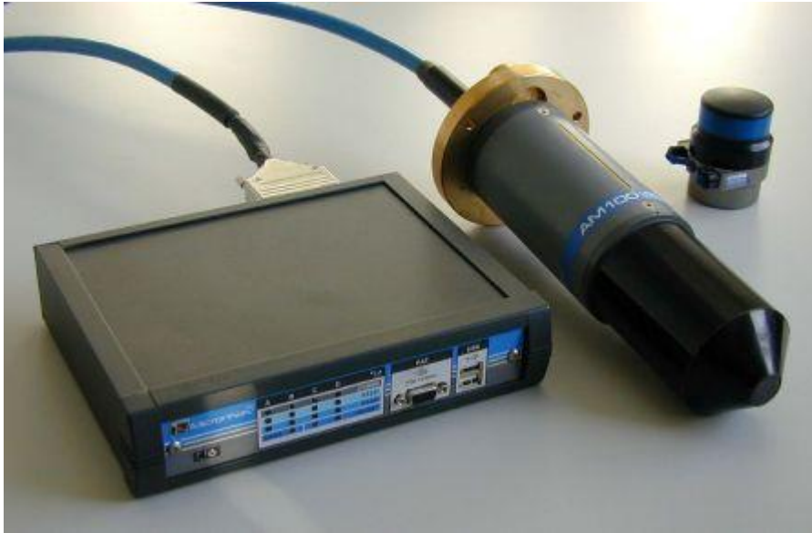
Fig.5. Underwater navigation system for the measuring module positioning.
