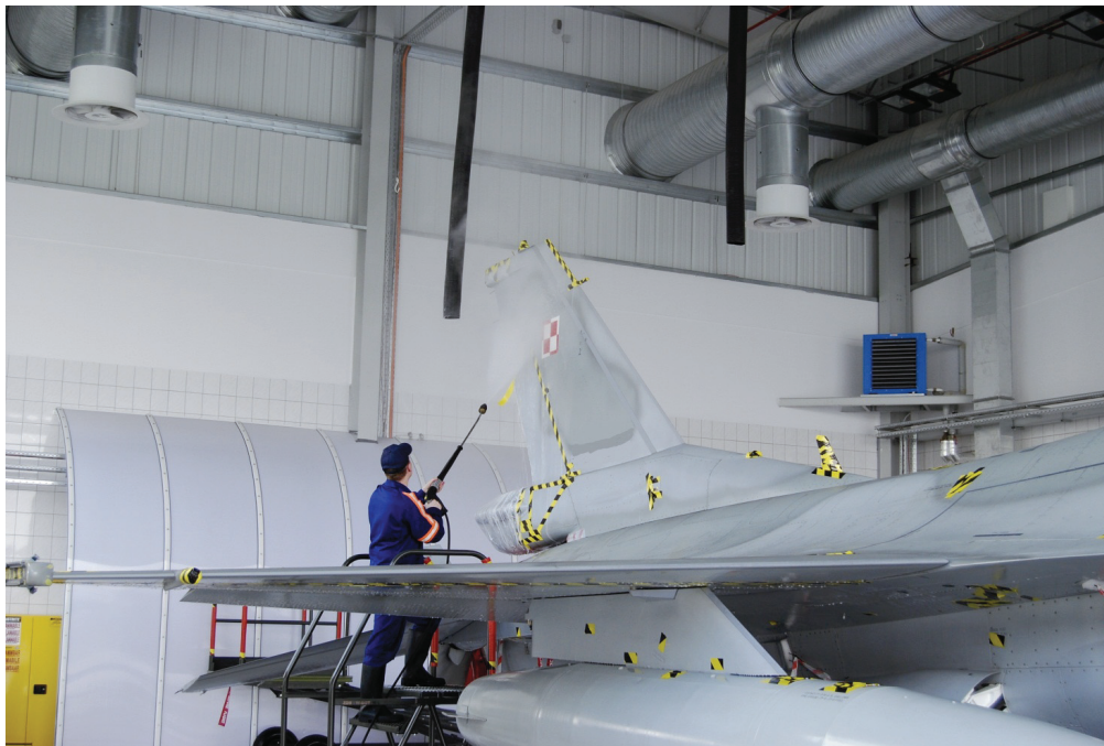
Fig. 1. F-16 vertical stabilizer cleaning process. Source: mjr pil. Adam Wójcik
