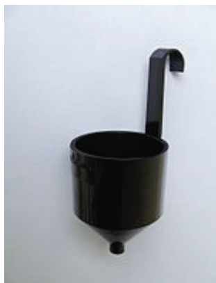
Fig. 3. Ford Viscosity Cup Source wikipedia.org
