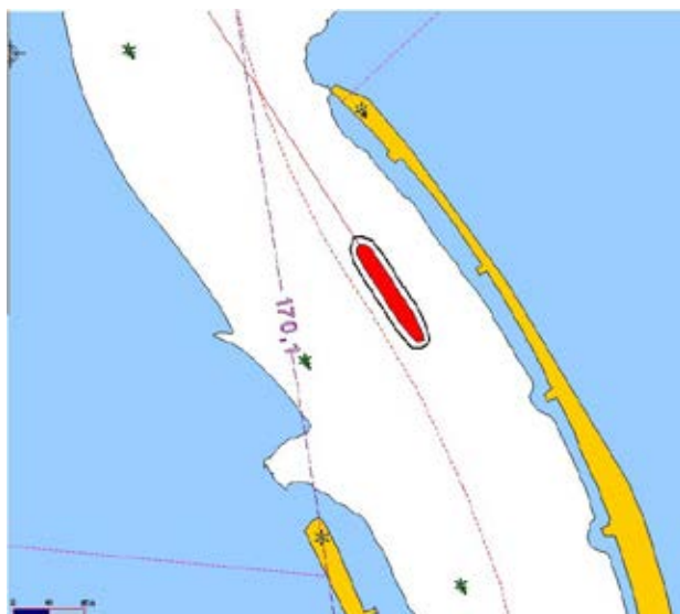
Figure 6. Presentation of a MVPA based on SBAS integrity data in an ECS display
