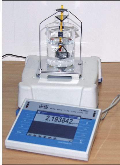
Fig. 2. Measuring stand for testing densities of metals and casting alloys by the immersing method
