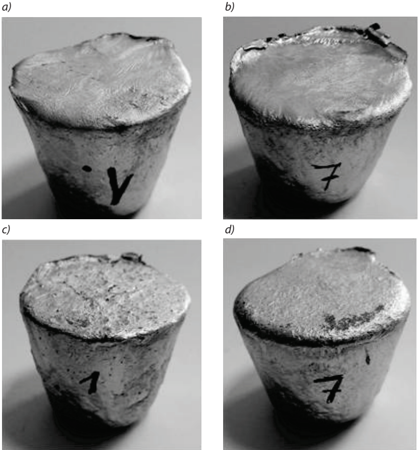
Fig. 5. Samples selected from individual melts solidifying under decreased pressure: induction thiristor furnace (samples a and b); silite furnace (samples c and d)
