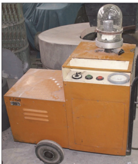
Fig. 4. Devices for assessing the gassing degree: a) ALU COMPACT II; b) GAS-METER
