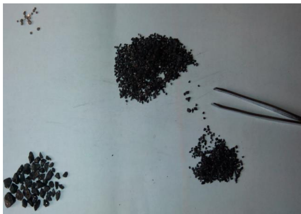
Fig. 5. (Picture left) Separation of the fraction of metallic from the slag: 1 - droplets of copper or a copper alloy drops separated from the slag; 2 - waste slag with copper droplets; 3 - greater fractions were re-fragmentation; 4 - waste slag
