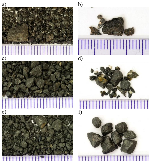
Fig. 7 a, b) Photographs gross fraction of the iron silicate slag-free copper by means of component A; c, d) Macroscopic photographs fraction of the iron silicate slag-free copper by means of component B; e, f) Photographs of gross fraction of the iron silicate slag-free copper by means of component D (scale division correspond with 1 mm)
