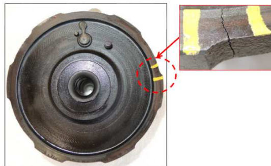
Fig. 2. Breakage of the flange of bearing housing
