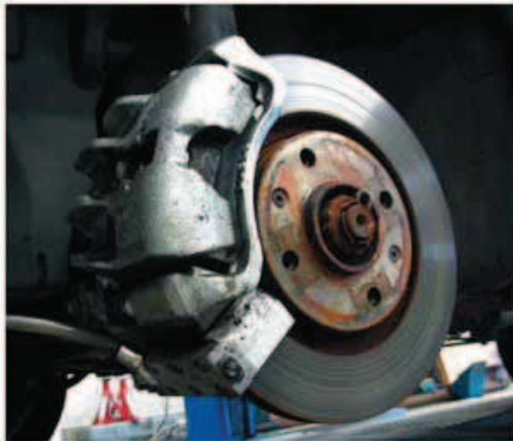
Fig. 3. Disc brake of the Citroen Berlingo vehicle provided with the dust emission reduction system
