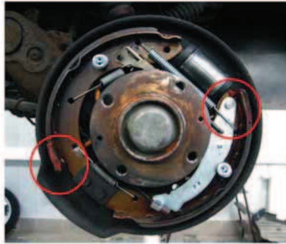
Fig. 4. Drum brake of the Citroen Berlingo vehicle provided with the dust emission reduction system (the red circles indicate the suction elements)
