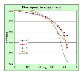
Figure 2. A comparison of simulated speed in straight runs in shallow water by four FMB training simulators, A, B, C and D (Gronarz, 2010)
