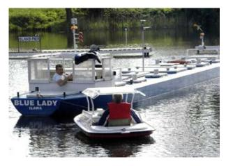
Figure 4. Manned tug working with model tanker
