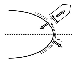
Figure 3. Schematic of the Coanda effect
