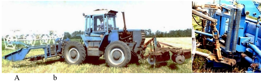
Figure 1. General view of the harvesting unit (a) and adapter (b) for attaching the header to the tractor
