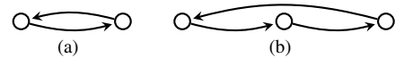
Fig. 5. Realization of the binomial: B_1 = 1 \pm \lambda^{-2} (a), B_0 = 1 \pm \lambda^{-3} (b).
