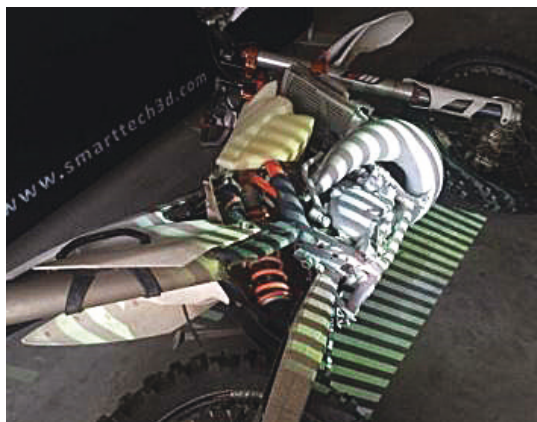
Fig.3. 3D scanning process
