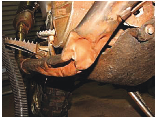
Fig. 2. Visible damage to the exhaust pipe
