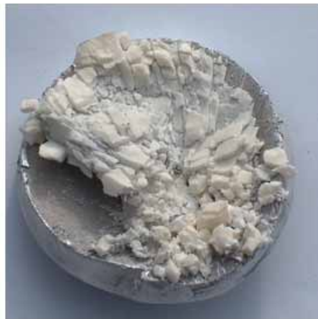
Fig.8b. Effects of firing the ŁPS shell with steel core and the energy of 3 kJ to 7020M alloy from the distance of 2 m - sample protected with ceramic \text{Al}_2\text{O}_3 of g = 6 \text{ mm}
