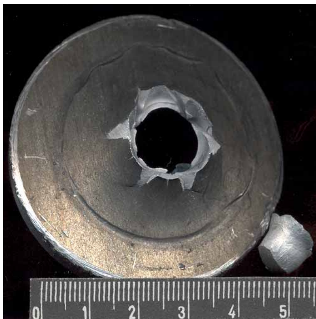
Fig.8a. Effects of firing the ŁPS shell with steel core and the energy of 3 kJ to 7020M alloy from the distance of 2 m - unprotected sample
