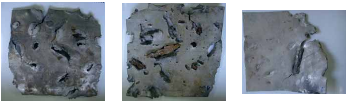
Fig.9. Effects of 7020M alloy sheet perforation (dimensions 300x3000): a) homogeneous g = 12 mm b) split ( w -inner, z -outer from the source of explosion, total thickness g = 2 \times 6 mm) after detonation of high explosive shell of OF412 type and calibre 100 mm with the contents of 1,4 kg of TNT, taking place at a distance of 0,6 m.
