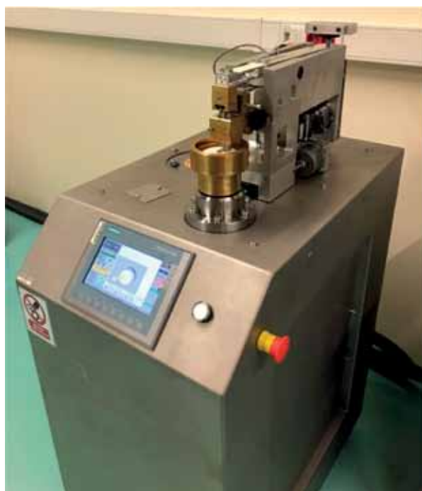
Fig. 1. Original ball-on-plane tribotester in one-way rotational motion manufactured at the Institute of Mechanical Technology at the Poznań University of Technology
