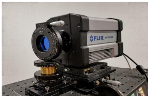
Fig. 2. Prototype of an LWIR division of a time polarimeter developed by FLIR Systems, Inc. (United States) [21].
