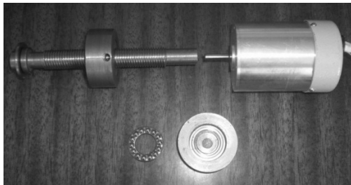
Fig. 10. SRM combining with reduction gear type of „screw set”
