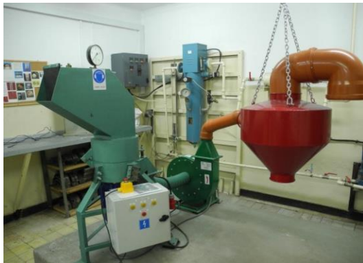
Fig. 1. Stand for processing composite materials acquired by the Gdynia Maritime University
