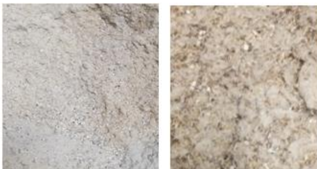
Fig. 2. Material sieved on a sieve, granulation: 1–1.2 mm, 2–3.0 mm
