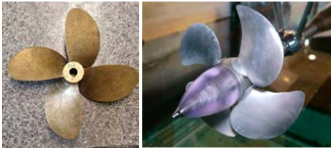
Fig. 1. P356 (on the left) and CP469 (on the right – prepared for the tests) propeller models
